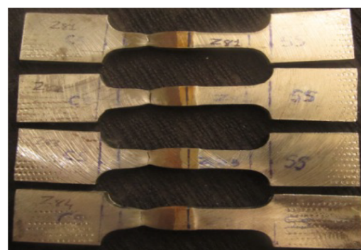
Fig. 2 a Dimensions of the tensile test specimen used in the present study. b N9 and c Z8 specimens. Both specimens failed on the CS side [1]
