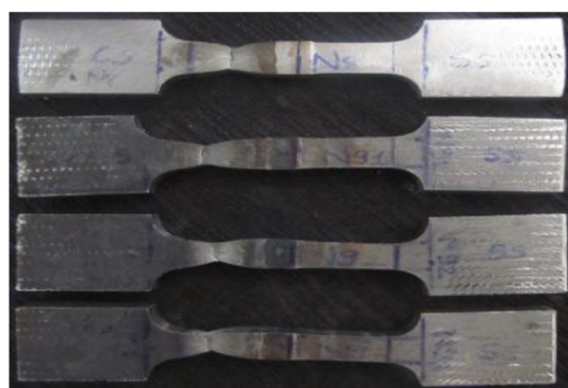
Fig. 2 a Dimensions of the tensile test specimen used in the present study. b N9 and c Z8 specimens. Both specimens failed on the CS side [1]
